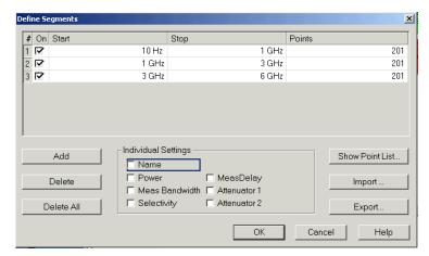
The *Define Segments* dialog contains a table to edit the individual segments of the sweep range. Sweep segments must not overlap, however, two adjacent segments can have one common point; see *Columns in the Define Limit Line table*.
