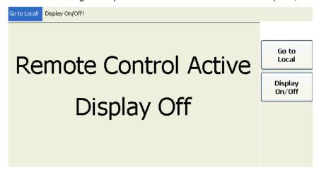
The two softkeys in the remote screen are used to modify or quit the remote state:
