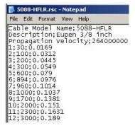
Pre-installed cable description files are stored in the  $C:\R_S\Instr\resources\Nwa\CableTypes$  directory. A new, user-defined cable type is stored under  $C:\R_S\Instr\user\Nwa\CableTypes$ .
