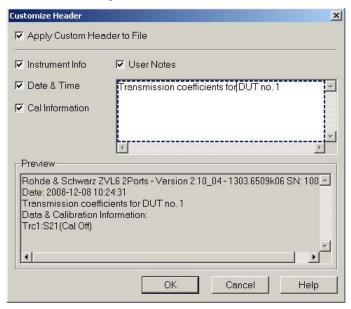
Select *Apply Custom Header to File* to insert the header in the *Preview* section at the beginning of the generated trace file. The *Instrument Info, Date & Time*, and *Cal Information* are generated automatically. The *Cal Information* contains the calibration for each exported trace. *User Notes* are additional, optional comments.
