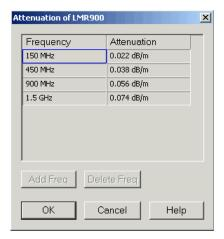
For user-defined cables, the *Frequency* and *Attenuation* columns in the dialog are editable. The frequency dependence can be defined in two alternative ways:
