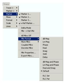
All marker formats are available irrespective of the measured quantity. The output values are calculated by a simple conversion of a complex measurement result, where the marker format defines the conversion rules. This flexibility in the calculation must be kept in mind when interpreting the results and physical units displayed; see also Measured Quantities and Display Formats.
