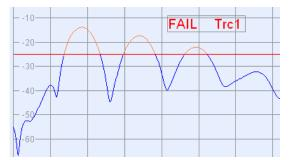
Remote control: CALCulate:TRANsform:DTFault:PEAK:THReshold
