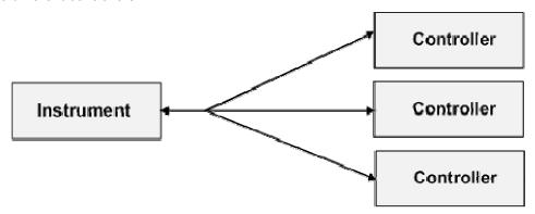
The controllers can lock and unlock the instrument for exclusive access. This regulates access to the instrument of several controllers.
