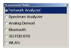
The spectrum analyzer mode and the supplementary modes require option R&S ZVL-K1.
