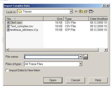
The loaded trace data is used to generate a memory trace which is coupled to the active data trace. *Import Data* corresponds to a standard *Open File* dialog with an additional checkbox:
