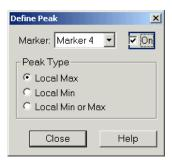
It is possible to select the peak type up to ten times for each trace and assign the selection to the markers no. 1 to 10.
