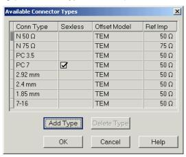
The list shows the available connector types with their name (Conn Type), polarity (Sexless) and reference impedance (Ref Imp). The Offset Model describes the mode of wave propagation in the transmission lines of the standards associated with the connector type. The buttons below are used to add and delete user-defined connector types. Deleting a connector type will also delete all calibration or adapter kits assigned to it.
