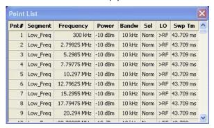
Points in inactive sweep segments (i.e. segments that are not switched *On* in the segment table) are not shown. The table provides a check of the settings made and can not be edited.
