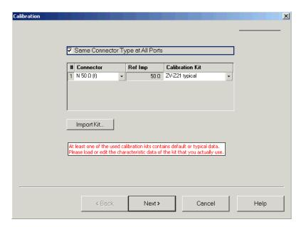
4. In the first dialog of the wizard, select the calibration kit (here: ZV-Z21) and the test port connector (here: N 50  $\Omega$  (f), corresponding to a male calibration standard), and click *Next*.
