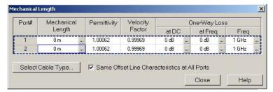
The Mechanical Length dialog contains the three editable columns Mech. Length, Permittivity ( $\varepsilon_r$ ) and Velocity Fact 1/sqrt( $\varepsilon_r$ ); see Offset parameters: Definition above. Permittivity and velocity factor are coupled parameters. The dialog provides the following additional control elements:
