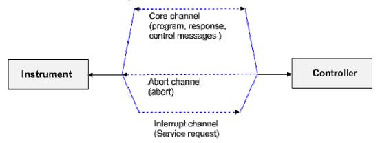
The number of controllers that can address an instrument is practically unlimited in the network. In the instrument, the individual controllers are clearly distinguished. This distinction continues up to the application level in the controller, i.e. two applications on a computer are identified by the instrument as two different controllers.
