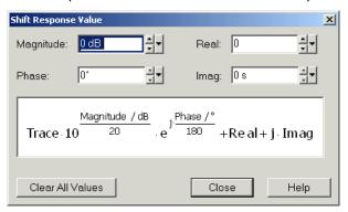
The units of the constants are adjusted to the format of the active trace. Setting all values to zero (Clear All Values) restores the original trace.
