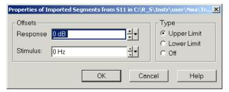
The dialog assigns common properties to all limit line segments generated by the imported trace.
