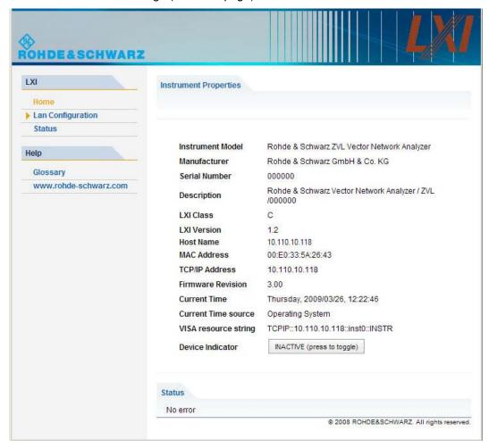
The instrument home page displays the device information required by the LXI standard including the VISA resource string in read-only format. The *Device Indicator* toggle button causes the LXI symbol in the status bar of the analyzer to blink (if active). A green LXI status symbol indicates that a LAN connection has been established; a red symbol indicates that no LAN cable is connected. The *Device Indicator* setting is not password-protected.
