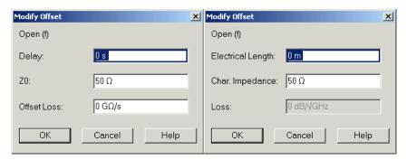
The offset parameters depend on whether or not the circuit model is defined in *Agilent Mode* (see *Add/Modify Calibration Kit* dialog):
