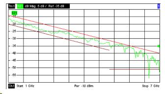
Display of the limit line and limit check are independent of each other: Hiding the limit line does not switch off the limit check.
