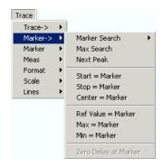
The functions in the upper section provide search functions to locate specific points on the trace.
