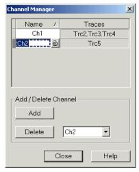
All existing channels of the current setup are listed in a table; see below. Below the table the *Trace Manager* provides the following buttons:
