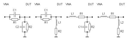
The following networks are composed of a shunt C or L (as seen from the analyzer port), followed by a serial C or L. They are named Shunt C, Serial C / Shunt C, Serial L / Shunt L, Serial C / Shunt L, Serial L.
