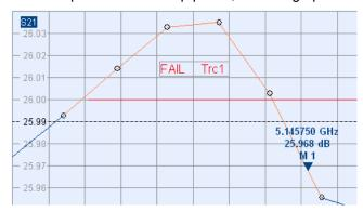
Remote control: CALCulate<Chn>:LIMit:STATe ON | OFF
