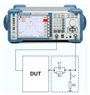
The idea of virtual embedding is to simulate the matching network and avoid using physical circuitry so that the analyzer ports can be directly connected to the input and output ports of the DUT. The matching circuit is taken into account numerically. The analyzer measures the DUT alone but provides the characteristics of the DUT, including the desired matching circuit. This method provides a number of advantages:
