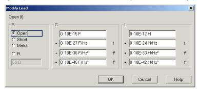
The circuit model for the load consists of capacitance C which is connected in parallel to an inductance L and a resistance R, both connected in series.
