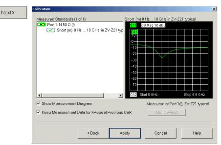
The next dialog of the calibration wizard shows that only a single calibration standard needs to be measured.
