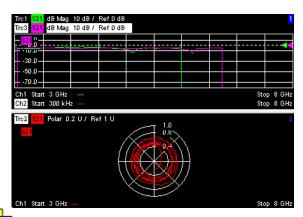
To vary the size and position of the two diagram areas, drag and drop the separating frames or use the *Split Manager*.
