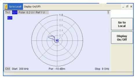
Switching on the display is ideal for program test purposes but tends to slow down the measurement. Therefore it is recommended to switch off the display in real measurement applications where a tested program script is to be executed repeatedly.
