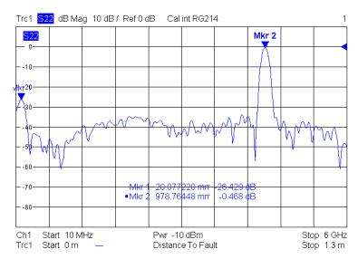
The parameters of the impulse response and frequency-domain representation are related due to the mathematical properties of the time-domain transform. In practice, this means that the sweep points may have to be adjusted to the length of the transmission line and the expected distance-to-fault:
