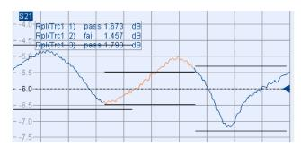
As a consequence of the limit line rules, the limit check will always pass a DUT if no limit lines are defined.
