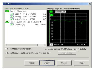
The dialog displays the list of measured standards compiled in the previous dialog. The list is complete: All standards must be measured to perform the selected calibrations.
