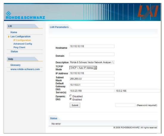
The *TCP/IP Mode* configuration field controls how the IP address for the instrument gets assigned (see also *Assigning an IP Address*). For the manual configuration mode, the static IP address, subnet mask, and default gateway are used to configure the LAN. The automatic configuration mode uses DHCP server or Dynamic Link Local Addressing (Automatic IP) to obtain the instrument IP address.
