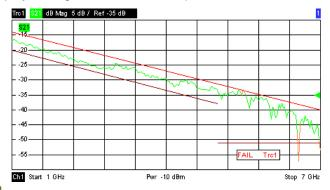
Limit check and display of the limit lines are independent of each other: With disabled limit check, the limit line can still be displayed, however, no display elements indicating a limit failure will appear.
