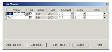
All existing traces of the current setup are listed in a table with several editable (white) or non-editable (gray) columns. Below the table the *Trace Manager* provides the following buttons:
