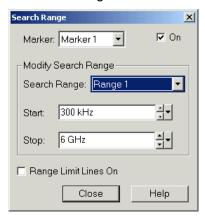
It is possible to define up to ten different search ranges for each setup and assign them to the markers no. 1 to 10. The input fields in the *Search Range* dialog are used to select the markers and define the associated search ranges:
