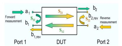
The S-parameters are the basic measured quantities of a network analyzer. They describe how the DUT modifies a signal that is transmitted or reflected in forward or reverse direction. S-parameters are expressed as  $S_{\text{out}>\text{c in>}}$ , where <out> and <in> denote the output and input port numbers of the DUT.
